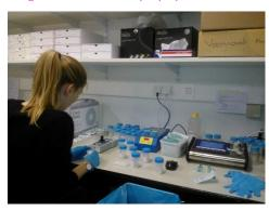
Fig. 2:: Emma determines vitamin A with the iCheck Fluoro
